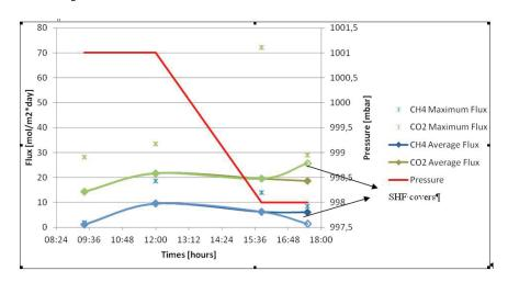
Fig. 2. Flux and pressure measured on the daily covers, field tests
