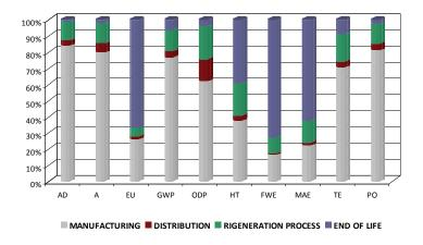
Fig. 2. The environmental impact potential (%) of LCA ILPO PUR shell of chairs life
