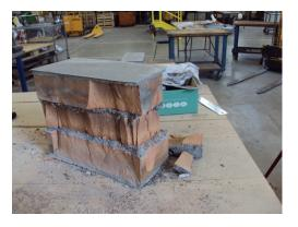
Fig. 2. A triplet after the compressive strength test
