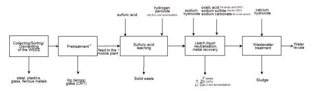
Fig. 1. Block diagram of the processes carried out in the HydroWEEE portable plant.
