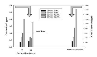
Fig. 1. Cr leaching as a function of curing time and compared to chromium in the waste
