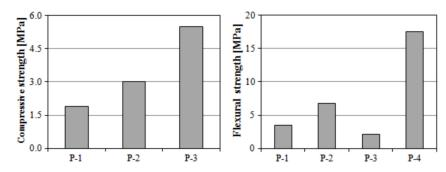
Fig. 2. Compressive and flexural strength of the panels
