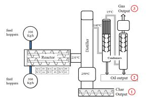
Fig. 1. Thermodynamic Cracking pilot plant worksheet (output: 1 char; 2 distilled oil; 3 incondensable gas).
