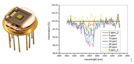
Fig. 1. Sensor developed (left) and measurement of acetaldehyde in  $N_2$  from 0 to 25 ppm in 5 ppm steps (right)
