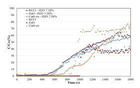
Fig. 4. Hydrogen sulfide removal for sorbent materials in dry and humid conditions
