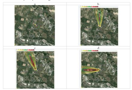
**Fig. 5.** Odour impact assessed by field inspection (a) vs. simulated by odour dispersion modelling considering different time ranges: 16-17 h (b), 17-18 h (c), 18-19 h (d)
