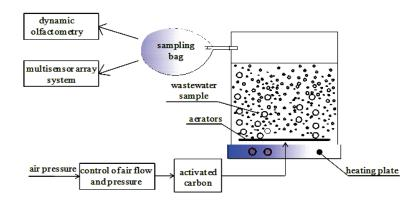
Fig. 1. Experimental setup used for odour emission sampling to OEC determination
