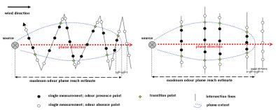
Fig. 1. Dynamic (left) and stationary (right) plume measurement
