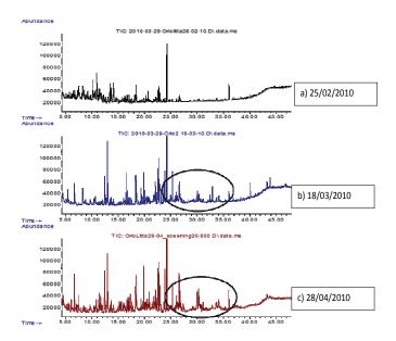
Fig. 3. TIC Chromatograms of the surface water of river Lambro after the oil spill (23/02/2010): the different chromatograms showed the evolution of the chemical fingerprinting in the months following the accident
