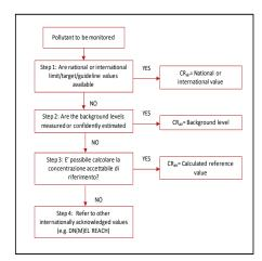
Fig. 1. Procedure flow sheet for VOCs assessment
