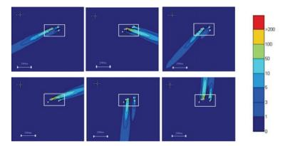
Fig. 2. Maps illustrating the individuation of the buffer zone considering the worst odour dispersion conditions for a landfill (case 2). The white rectangle delimits the plant perimeter; the white points are the odour sources. In all maps, since the isoline of 50 ou/m³ falls within the plant perimeter, the buffer zone overlaps with the plant boundaries.
