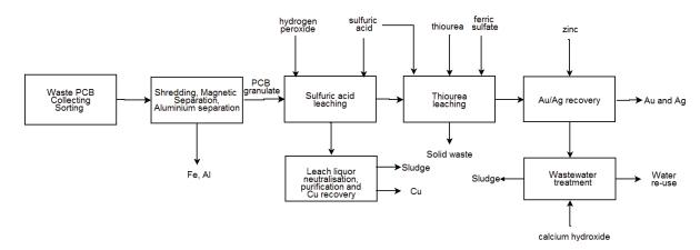
Fig. 2. Block diagram of the process carried out in the HydroWEEE portable plant aimed at metal recovery from PCB granulate
