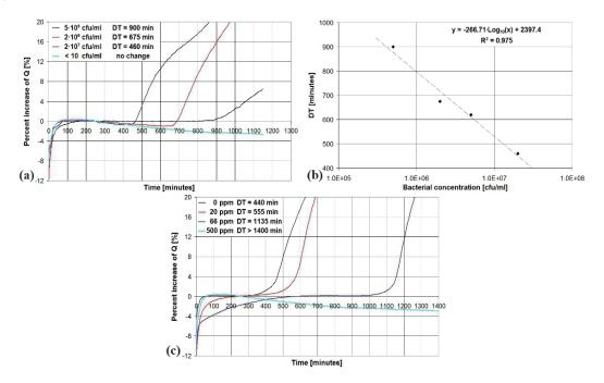
**Fig. 2.** Percent increase of Q vs. time for samples featuring different values of bacterial concentration (a). Scatter plot of the measured DT vs. bacterial concentration of the tested samples (b). Percent increase of Q vs. time for a sample inoculated with different amount of biocide (c)
