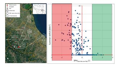
**Fig. 1.** Left: Location of the Ridracoli reservoir (triangle) and of the rain gauges used for the analysis of the precipitation regime of the period (1945-2010); simplified scheme of the Ridracoli Reservoir supply system. Right: Summer deficit plotted vs the winter precipitation represented by the SPI4<sub>Nov-Dec-Jan-Feb</sub>. Green and red shaded areas represent unconditional lack of deficit and unconditional presence of deficit, respectively
