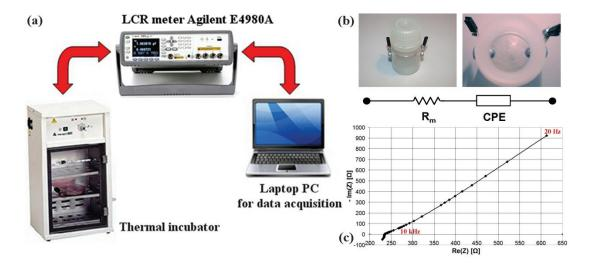
Fig. 1. Measurement setup used in the study: (a). Sensor hosting the sample under test and electrical circuit used to model the electrical response (b). Nyquist diagram for a sample under test (c)
