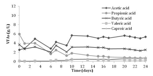
Fig. 2. VFAs concentrations observed during PBBR operation
