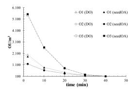
Fig. 4. Comparison of predicted and measured odor concentrations during the OEC stripping test.
