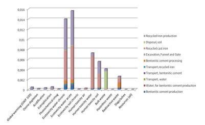
Fig. 2. Impacts of the Permeable Reactive Barrier, operation and disposal processes in the different impact categories (including long-term impacts) [Pt]
