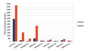
Fig. 1. VFAs concentration in second step influent end effluent
