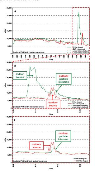
**Fig. 1.** Schematic representation of the method used for subtracting the internal sources (A: indoor, green, and outdoor, red, PNC profile in a summer day; B: magnified part of A with internal and external source related peaks; C: resultant profile after subtraction of internal sources)
