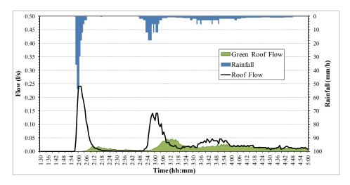
**Fig. 3.** Monitoring results for the rainfall event collected on 20/08/2013; comparison between impervious roof and green roof flows
