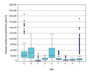
Fig. 1. Box plot of PNC (1 min averages) measured in several microenvironments: R1 WIN MODE (A); R2 WIN MODE (B); R1 AC MODE (C); R2 AC MODE (D); kitchen during cooking (E); living room (F); bedroom, night (G); office building (H); outdoor all measurements in 31 sites (I).
