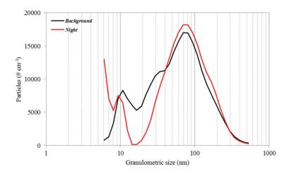
Fig. 1. Particle profile during background and nighttime measurements.
