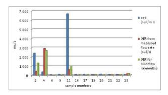
Fig.3. OER of the punctual odour emission sources of the plant
