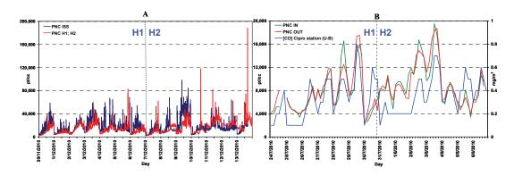
**Fig. 2.** A: time series of outdoor PNC measured in the two sapling sites (Home 1, Home 2) and in the ISS reference station; B: comparison between indoor/outdoor PNC and carbon monoxide concentration measured in a urban background station belonging to the air monitoring network of Rome
