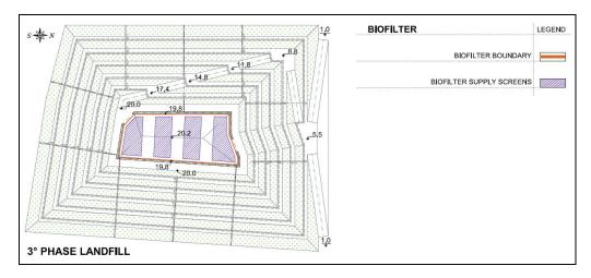
Fig. 1. Schematic plan of 3<sup>rd</sup> phase landfill with identification of biofilter boundary and supply screens
