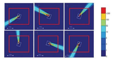
Fig. 1. Maps illustrating the individuation of the buffer zone considering the worst odour dispersion conditions for a landfill (case 1). The white rectangle delimits the plant perimeter while the red one individuates the buffer zone perimeter; the white points are the odour sources. In all maps, the buffer zone is defined on the bases of the isoline of 50 ou/m<sup>3</sup>.
