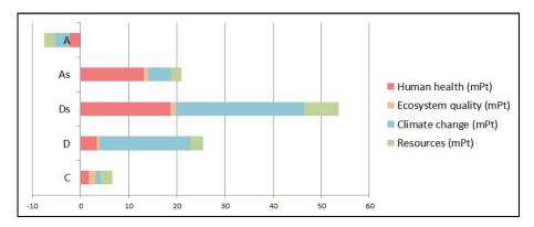
**Fig. 1.** Comparison between sludge recovery/treatment systems (IMPACT 2002) L = Landfill, A = land Application, s = stabilization, C= Composting
