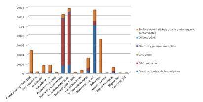
$\textbf{Fig. 1.} \ \, \textbf{Impacts of the Pump \& Treat System, operation and disposal processes in the different impact categories (including long-term impacts) [Pt]}$
