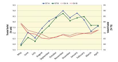
Fig. 1. Total (ST) and volatile (SV) solid variation over the year in the two digesters (A and B)
