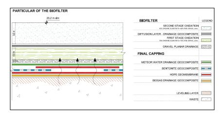
Fig. 2. Schematic section of the oxidation biofilter
