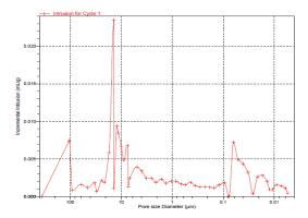
Fig. 1. Pore size distribution versus mercury intrusion volume for the sample containing 75 wt % of glass
