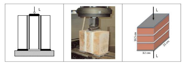
Fig. 1. Scheme of the shear and compressive test and a triplet during the testing
