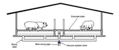
Fig. 1. Fully – slatted floor with vacuum system (BREF, 2013)
