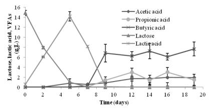
Fig.1. Lactose, lactic acid and VFAs concentrations in microcosms during the batch experiment
