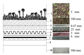
**Fig 1.** Extensive green roof with sedum plants and twin reference roof; Layers for green roof (\* Elements constituting the SEIC green roof system): 1. Extensive vegetation – Sedum; 2. SEIC extensive substrate - growing medium; 3. Optional anchoring system for tilted roofs; 4. MediFilter MF1 - filtering mat; 5. MediDrain MD 25 – drainage element; 6. MediPro MP300 - root protection fabric; 7. Waterproofing root barrier membrane; 8-9-10. Structural elements
