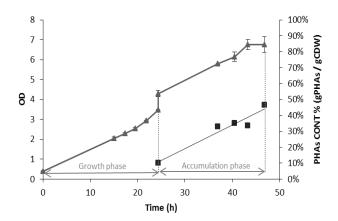
Fig. 2. Biomass (triangles) and total PHAs content (squares) during the sequential batch experiment. This is for an accumulation culture media containing 25% of  $OMW_{Acid}$
