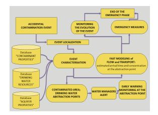
Fig. 2. Scheme of the best practice protocol for the emergency management of groundwater contamination
